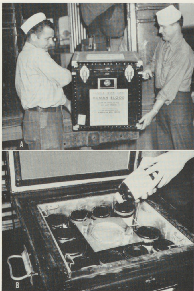
FIGURE 184.—Trunk type of insulated container developed for Army by Hollinger Corp. during Korean War. A. Closed. B. Open, loaded with ice and blood and ready for shipment. Note that bottles are upside-down, so that blood cells will settle in the top.
