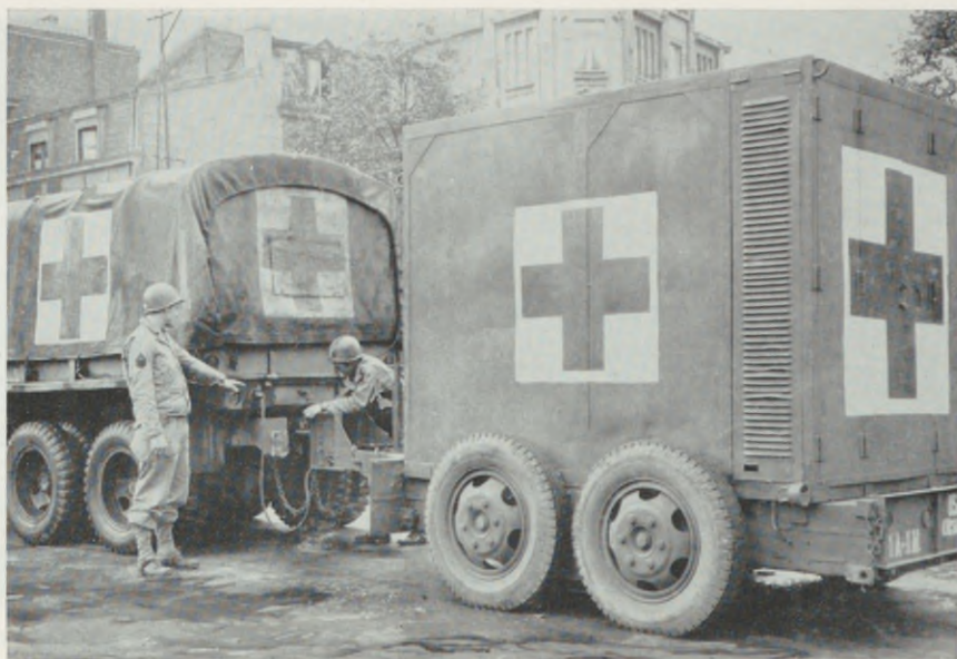
FIGURE 124.—Delivery vehicle with 80-pint refrigerator in truck body. Behind this vehicle is 1,000-pint mobile refrigeration truck of Detachment A, 152d Station Hospital, First U.S. Army, Belgium, October 1944.
